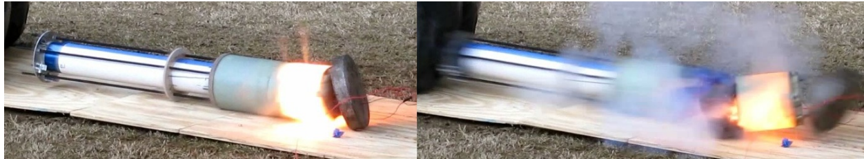
Figure 11: Drogue Chute Test time t = 0 and time t = +\frac{1}{30} sec
