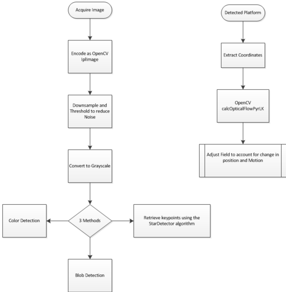
Figure 62. A.P.E.S. Detection, Characterization, and Control Process Flow Diagram.
