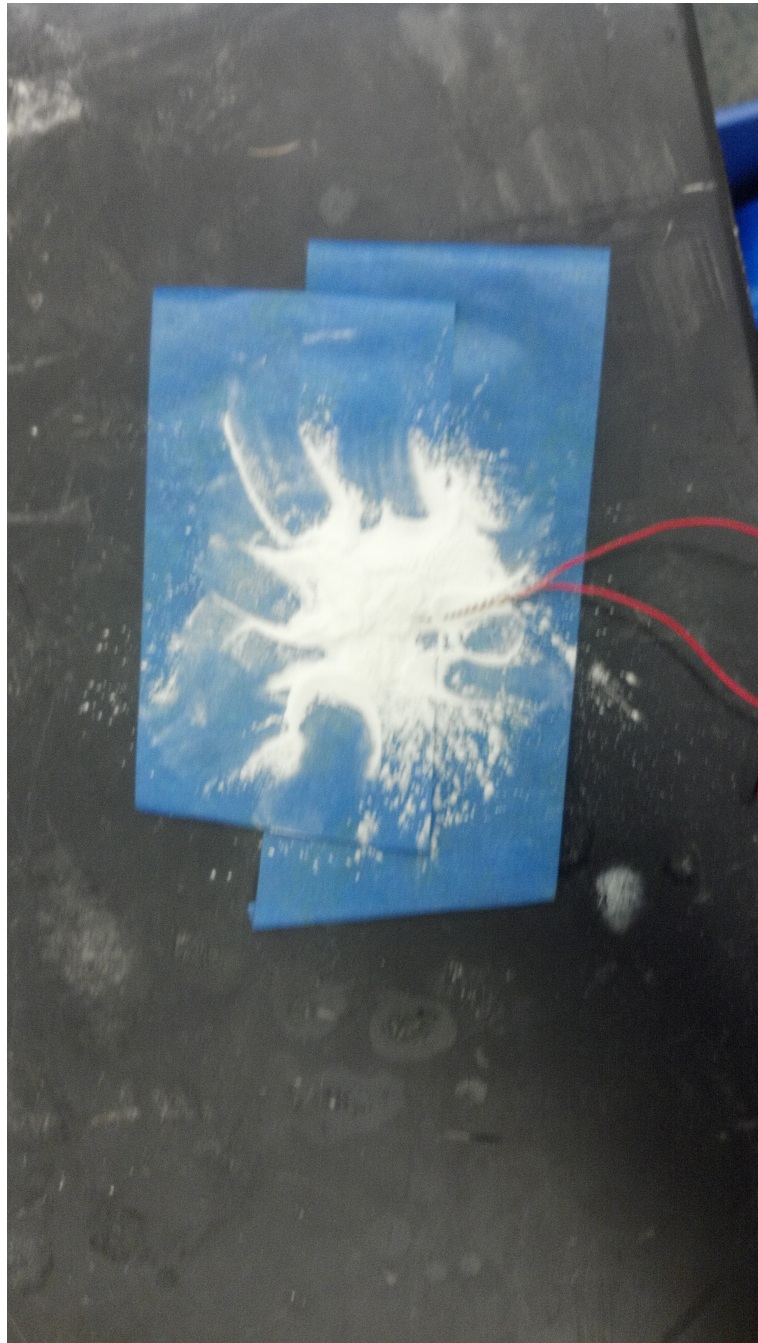
Step 3.3: Pour pre-measured black powder on top of ejection charge
