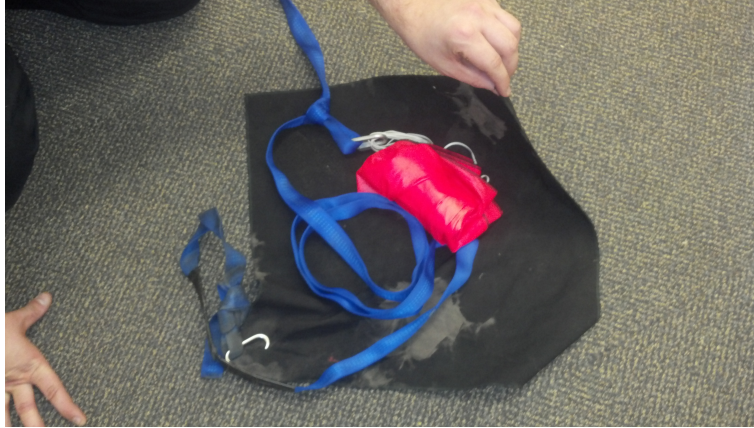
Step 1.8: Place the folded parachute onto a NOMEX cloth
