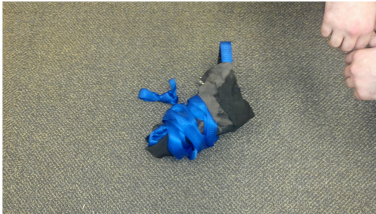
Step 1.9: Fold NOMEX cloth around the parachute
